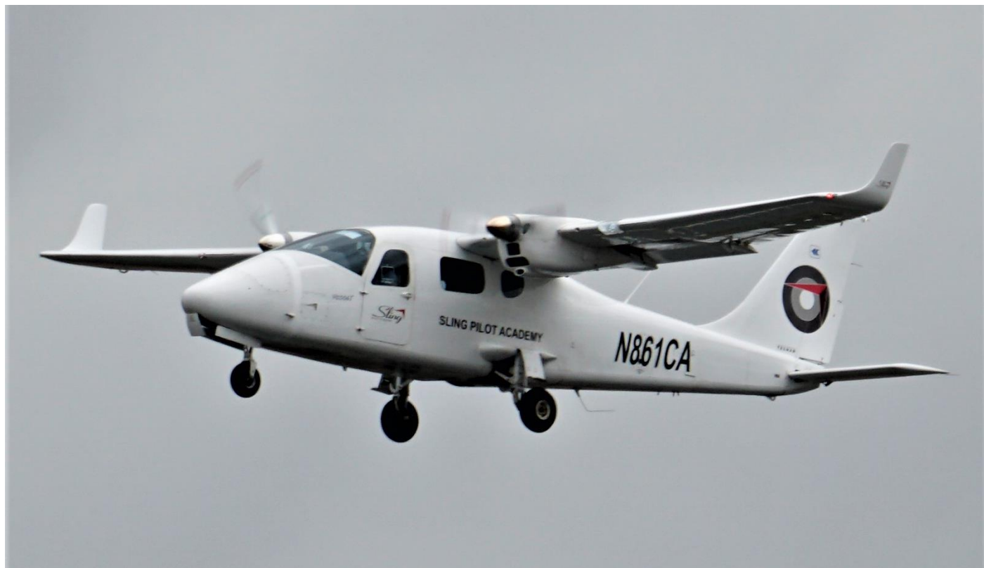
It's a Tecnam P2006T from Italy. Four seats and two 100 hp Rotax 912S engines. It's being marketed as a low-cost twin-engine trainer. Photo by Jim MacKinnon. 10/10
