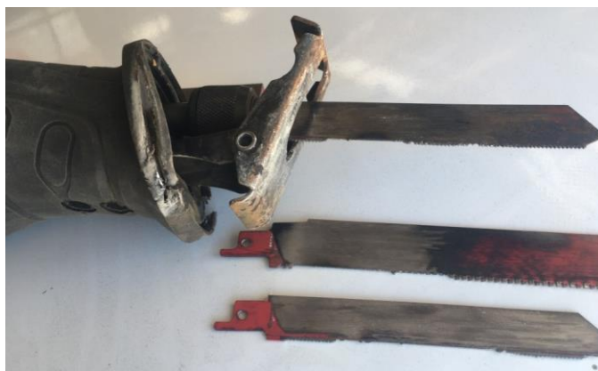
Chopping up a hangar is hard on sawblades. The crew went through three carbide blades while reducing the carcass to scrap and trailer material.
