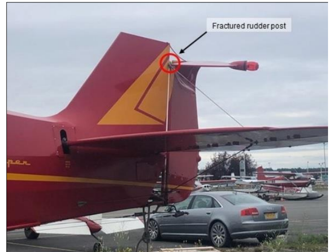
The following pictures show the fractured rudder posts of the two Pipers.
