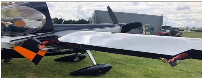
G-EDGY after landing, showing inboard hinge with section of aileron still attached and the distorted outboard hinge
