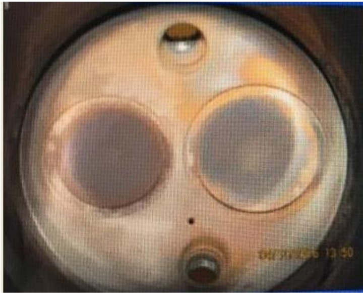
Cylinder head running 100 LL. Note deposits.
