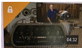
Setting VW Engine Valve Clearance March 16, 2020 | 694 Views Tim Hoversten from the EAA staff demonstrates how to set valve clearance on the VW engine.
