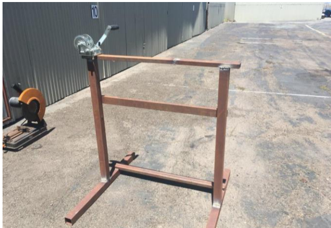
Ryan's winch stand, constructed to ease the Katana off the semi-trailer. There's a photo of it in action on p. 6.
