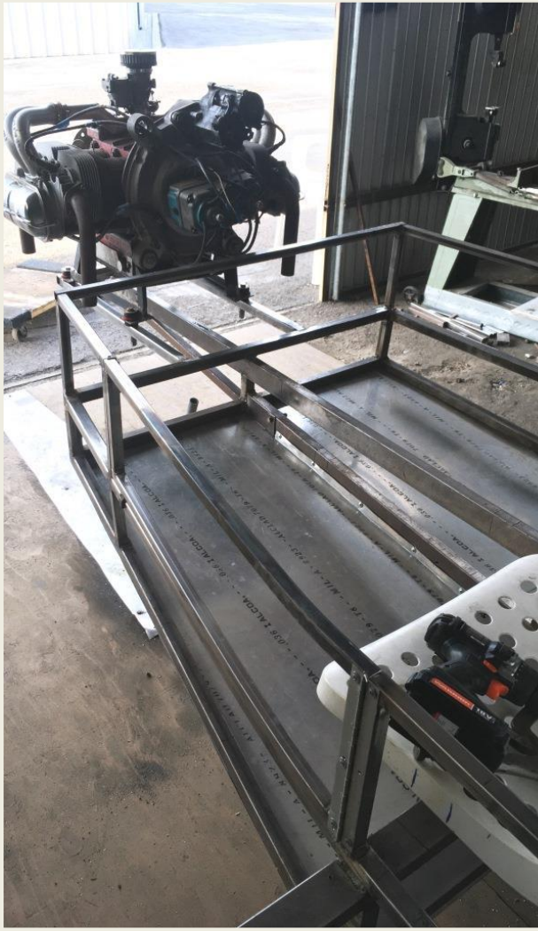
▲ Fabricated a basic floor using sheet metal.
