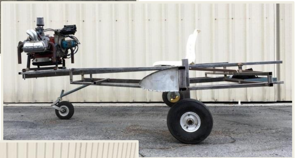
◀ Engine added back to plane in a slightly new position. Exhaust now points down. ▼
