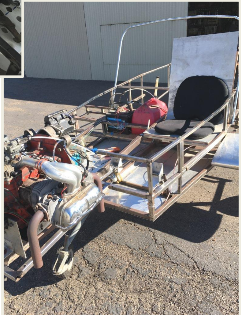
Started customizing the pilot's seat. Installed wiring to fuel tank for easier temporary starting. ►
