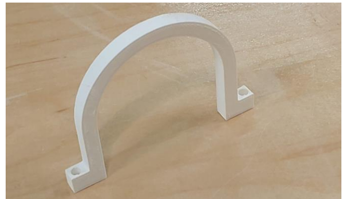
Figure 10. Hold-down clamp fresh from the 3d printer. All that remains is to see if it fits. If it doesn't, it's easy to modify the CAD design and print another one.
