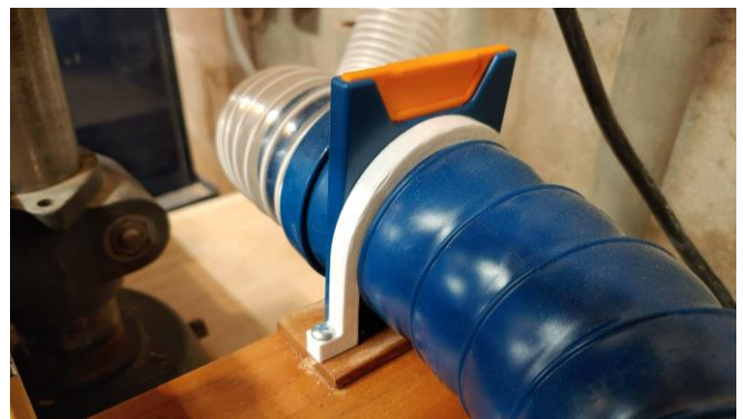
Figure 11. Completed hold-down clamp in place. This clamp mounts to my drill press auxiliary table to stabilize the Loc-Line system I'm using for dust collection.
