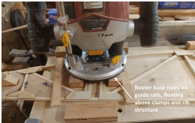
Figure 4. Router Fixture in Action. In use, the router base rides on the fixture guide rails, floating above the clamps and rib structure. This feature eliminates interference from rib structure and hold-down clamps.
