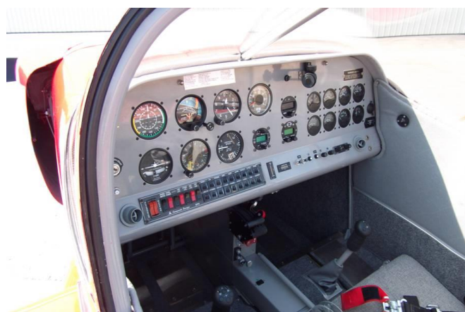
Final all-electric instrument panel optimized for VFR operation.
