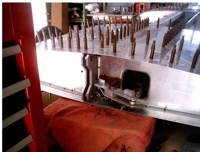
Two steel fittings that mate with a single steel fitting on the outer wing. Also shown is one of the two mating bell cranks. There is a bell crank on the outer wing.
