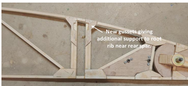
Figure 6. New Gussets Installed. This new gusset design was suggested by Dave Cooper, owner of Team Mini-Max in Niles, Michigan.
