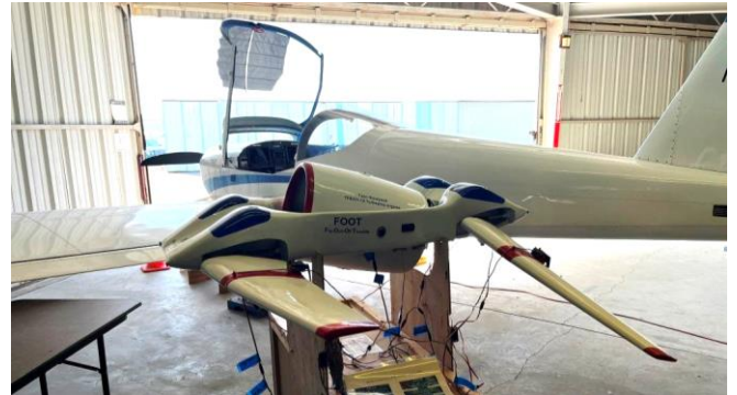
FOOT model in Hangar 3 next to Gert's RV-10. The double fuselage allows free airflow through the thrust assembly.
