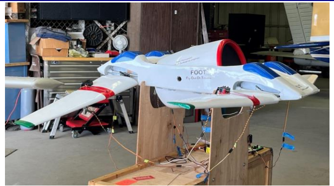
FOOT model in its cradle. Engine pod transitioning to horizontal flight configuration
