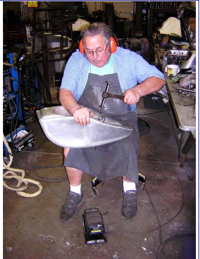
Rob taps in an adjustment to an aluminum fuel tank.
