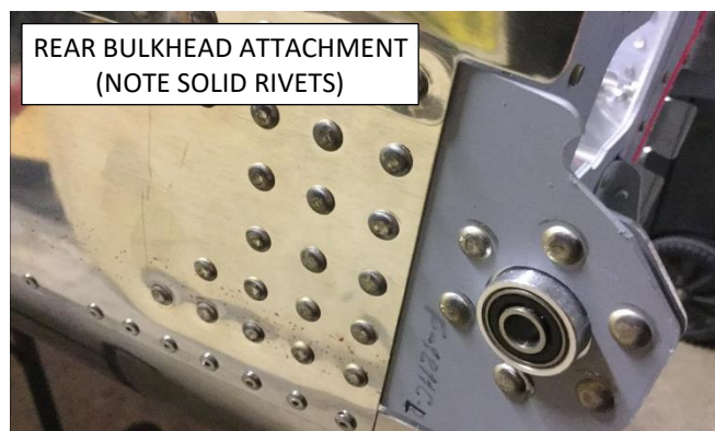
STABILATOR ATTACHMENT BULKHEAD
