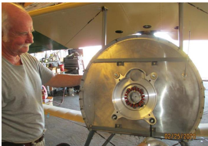
Meanwhile, Gene Hubbard is hard at work scoping out location of the magneto and starter clearance holes in his firewall.
