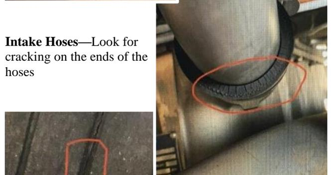
**Intake Hoses**—Look for cracking on the ends of the hoses
