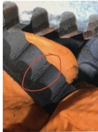
**Alternator Belt**—Look for cracking between the teeth
