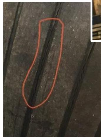
**Tires**—Look for cracking in the tread grooves.
