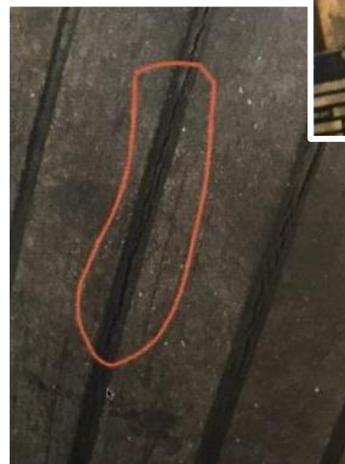
**Tires**—Look for cracking in the tread grooves.
