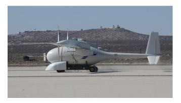
On its first flight, the Phantom Eye climbed to an altitude of 4,080 feet and reached speeds of 62 knots (71 mph/115 km/h). However, when landing, the Phantom Eye's landing gear dug into the Edwards Air Force Base lakebed and broke. The Boeing team says it has now improved the aircraft's landing system, while also improving its autonomous flight systems and upgrading its engine oil pumps.
