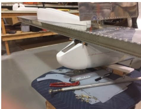
Fitting of tail cone
