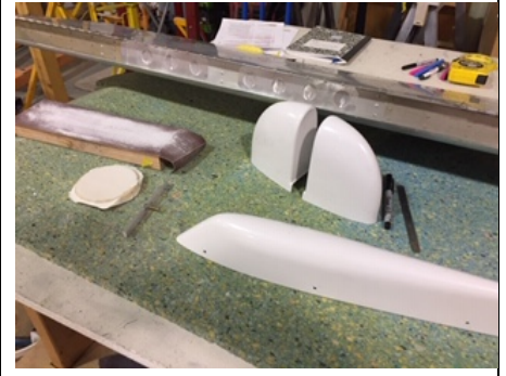
ABS parts being shaped and fitted on control surfaces
