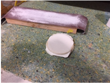
Small composite work for an inspection hole
