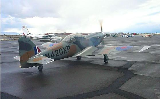
Vern bought the aircraft in 1997 as a partially constructed two-place tandem plans kit and spent the following fourteen years completing the project---he finally had his first flight in 2010! It holds 60 gal of fuel with a burn rate of 12-13 GPH, a cruise speed of 210 MPH, an empty weight of 1,860 lbs. and gross of 2,600lbs. It is currently for sale with an asking price of \$250,000.00 and total tach time of 37 hrs.
