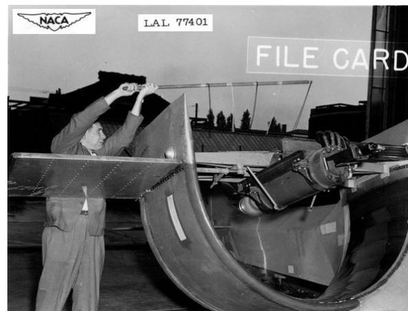
With its propeller blast channeled through a semi-circular wing, an infinite CL was claimed. Such high lift would give the ultimate in STOL performance; shortening approach and departure distances. Aerodynamically, the high lift would enable reduced wing size, weight, and complexity, enabling enhanced low-speed safety and control.
