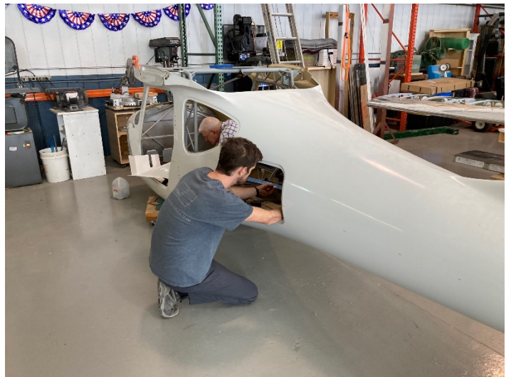
Working on and installing cable tunnel (Kellan at work)
