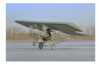
Ding Shilu is an automobile mechanic in China. His 285-pound, three-engine homebuilt aircraft incorporates a short span, low aspect ratio, deeply cambered, flat-bottom wing with flat ailerons trailing behind the inboard portions of the trailing edge. Nearly two dimensional tail surfaces attach to a truss structure extending behind the pilot's seat, which sits below the wing on tricycle gear.
