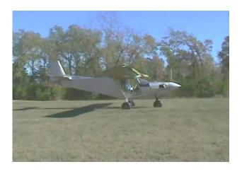
This is Scott Ehni's custom Zenith CH701 airplane (that he scratch-built from plans) powered by the lightweight Garrett JFS 100-13A Turbo shaft engine, putting out at least 90 BHP at a prop speed of 3,100 rpm and burning about 12 gph. The small APU works on almost any liquid that will burn. The best off-airport fuel choice is a mix of diesel and unleaded regular gas, as it burns a bit cleaner.
