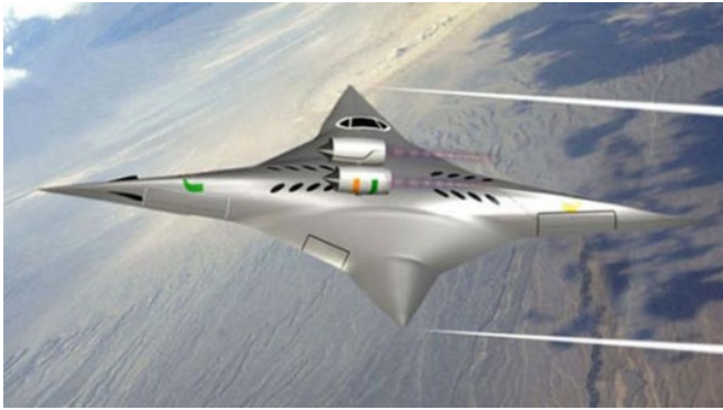
The supersonic bi-directional flying wing aircraft in high-speed configuration ...
