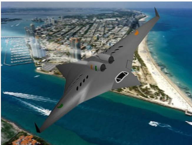
The supersonic bi-directional flying wing aircraft in low-speed configuration ...
