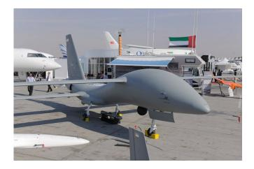
Based in Abu Dhabi, Adcom Systems' has forged a reputation for taking innovative approaches to UAV and aerial target design, and the United 40 does not disappoint due to its tandem-wing layout and dramatic S-shaped fuselage.
