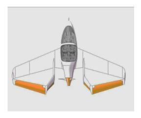
Synergy's signature shape, features an innovative "double box tail" - as opposed to a box wing, which have been known to have safety issues. The double box tail creates extremely low induced drag - described by McGinnis as the "glider-like efficiency of a 46-foot wingspan packed into a much stronger 32-foot package."
