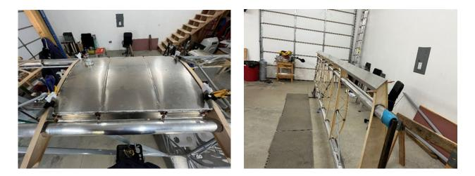
Last weekend I removed the wings so I could begin fitting up the flaps and ailerons.
