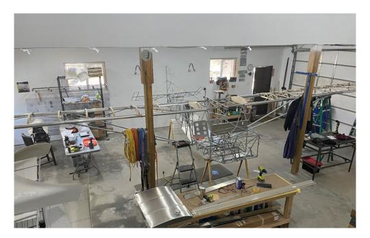
The most recent work was fitting the fuel tanks to the wings and fitting the wing trailing edge.
