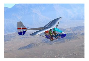
Although the aircraft is equipped with a small electric motor to fit into the FAR Part 103 category (allowing for flight without an FAA pilot certificate), all initial flight tests were conducted as a pure glider without any of the drag reduction enhancements and without the use of power. Flight testing will continue into the spring in different configurations: pure glider, glider with a single-engine electric sustainer motor, 40-hp single-engine, twin-engine, and tri-motor.
