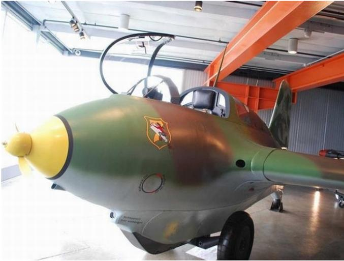
The Komet was a rocket-propelled fighter, built specifically to destroy high-altitude bomber planes. Unfortunately, its fatal flaw was its Walter rocket motor, which had a tendency to explode mid-flight. It was, however, a breakthrough in technology at the time. The model seen here is only one of a dozen Me-163 fighter planes left in existence.
