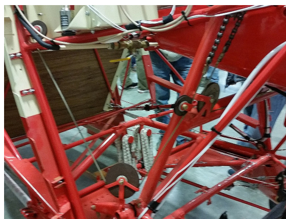
Landing gear bungees and control lines
