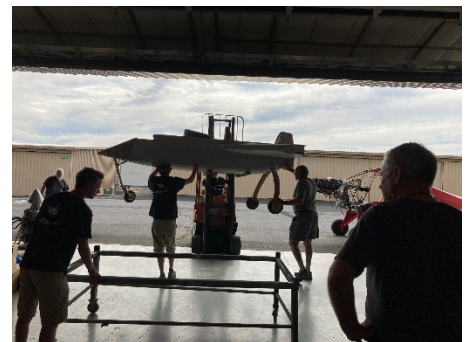
Below: Removing the wing to move the Varieze from the hangar
