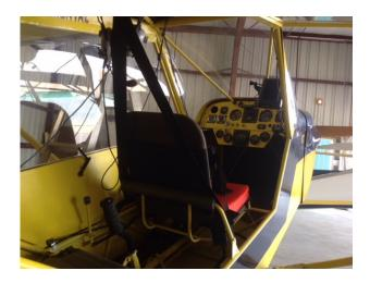
It's a very low time plane, hardly any on plane and a touch over 100 on motor. It's the early solid lifter Jabiru 2200 so it doesn't have the thru-bolt problems some of the later hydraulic lifter ones did. Good motor.
