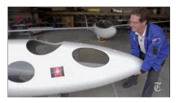
In the end, all will be painted a reflective white to stop the sun from heating the parts enough to weaken the epoxy. (Inside the cabin, though, the air will be near freezing.)
