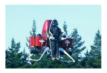
Flight tests of the company's 12th and latest prototype are underway and being flown unmanned to expand the low-altitude envelope as Martin modifies the engine, adding a balance shaft to reduce vibration inherent in the 200-hp. V4 two-stroke which powers a pair of ducted fans to provide both vertical thrust and flight control. Martin is aiming for a maximum speed of 40 knots. Empty weight manned is 400 lbs and maximum takeoff weight 720 lbs, for a payload with full fuel of 220 lbs.
