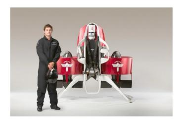
Altitude is limited to 3,000 ft. by microlight rules but, in May 2011, the P11 was flown unmanned to 5,000 ft. to show the machine could fly out of ground effect and "prove it's an aircraft".
