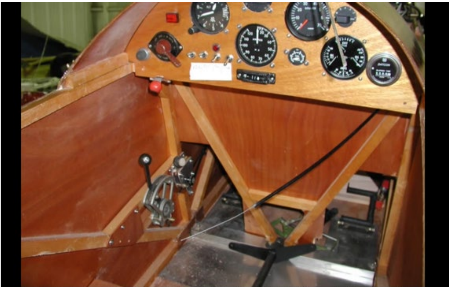
from left to right: Start button, A-9 mag and battery switch, red knob below is choke, red button above is battery warning light, altimeter, 4 switches are ignition, avionics, fuel pump w/ warning light and strobe, ASI, Compass, fuel press, tach, quad gauge is amps, oil press, oil temp, and CHT with rotary switch with probe on each cylinder. Hobbs meter. Below on left is throttle and small control ahead is carb heat. The cable hanging down not connected is fuel shutoff.
