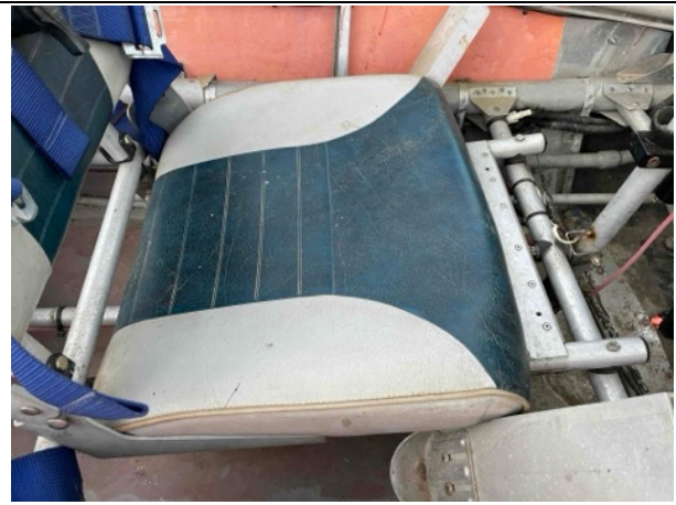
Front seat rubbing the rear rudder pedals? That's a definite "must fix"!
