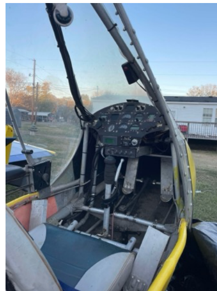
Front seat rubbing the rear rudder pedals? That's a definite "must fix"!
