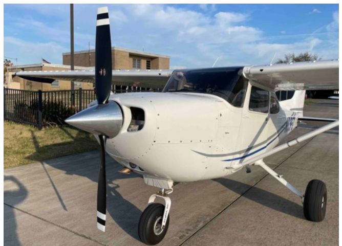
Does anything look strange about this 172? (Big ass front fork, a cowl flap, constant speed prop, and vortex generators. That's pretty cool.)
