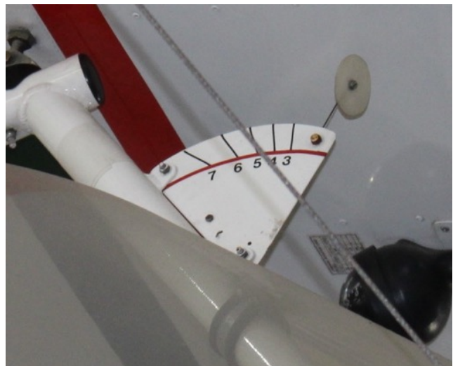
“Balerit’s” Single Moving Part Airspeed indicator
