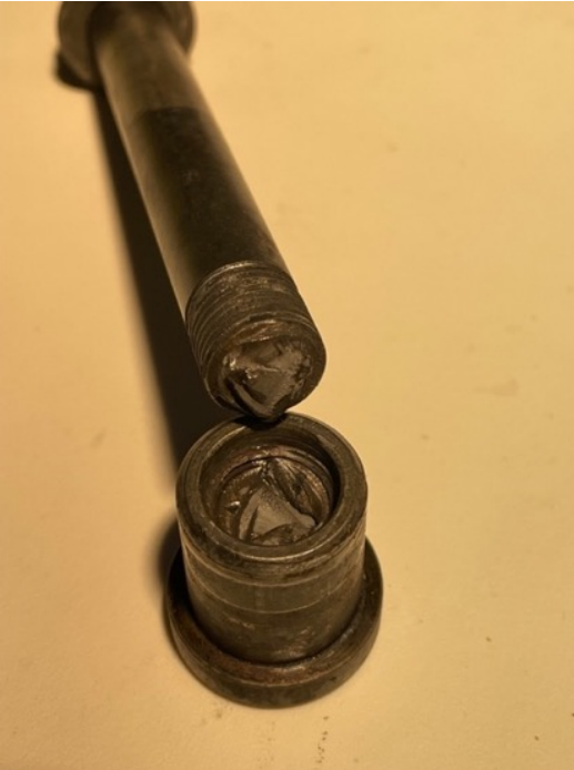
Fractured bolt and companion bushing/nut.
