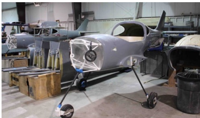
Lightning XSs' awaiting paint and Continental Titan engines.
