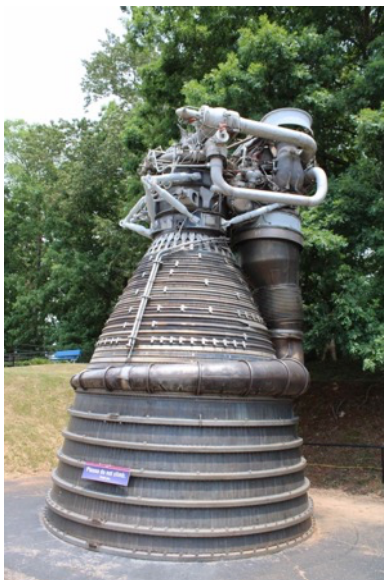
The Rocketdyne F-1 engine for the Saturn V. This thing consumed 1350 gallons of kerosene a second! (Wow. How far could you drive your diesel car/truck on 1 second worth of fuel for this beauty?)
