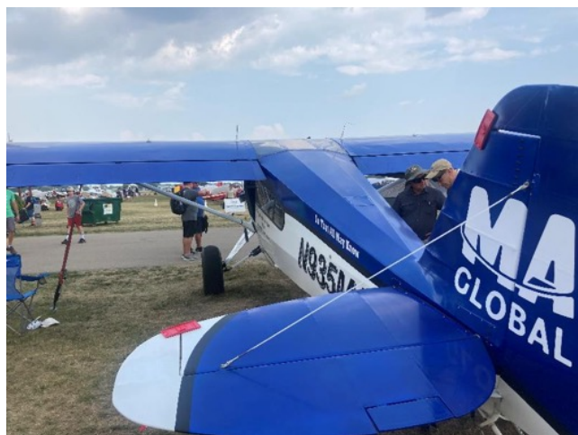
Backside of the Bearhawk Model 5. The new flap design goes all of the way to the wing root.
