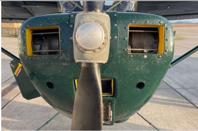
Hum. Notice anything missing? (No intake louvers on the rods.)
