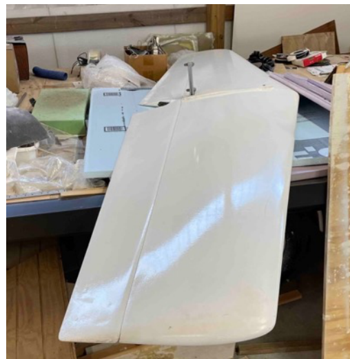
ASK-21 Stab. See that single bolt? That’s what holds it on folks.
