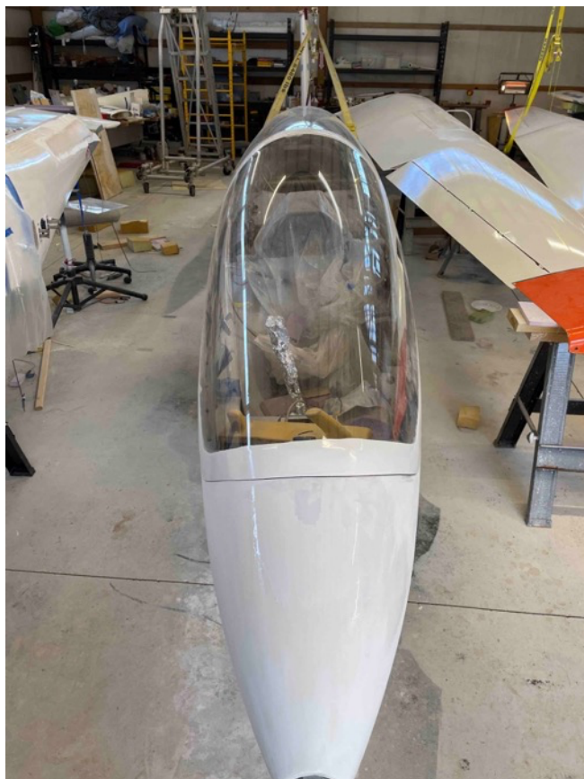
DG-1000 fuselage with (we were told) a scratch-built canopy
