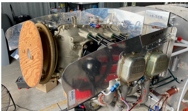
Yes, cooling baffles are definitely needed.
