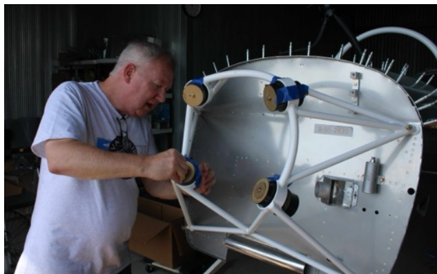
See, if we tape all these vibration isolators (A.K.A. "rubber doughnuts") in place, we should just be able to bolt the engine on.
