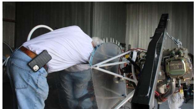
Randy's good side? No, attaching nuts to the back of the engine mount bolts!
