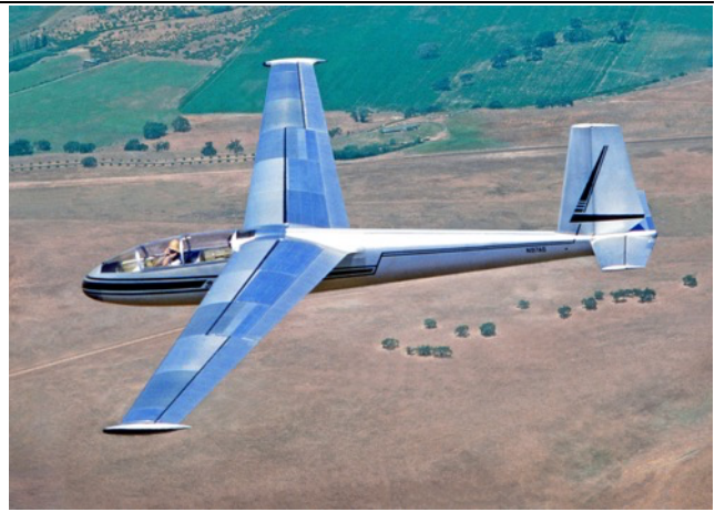
Blanik L-13 Sailplane. (EEZ: Note forward swept wings and unusual wingtips.)
