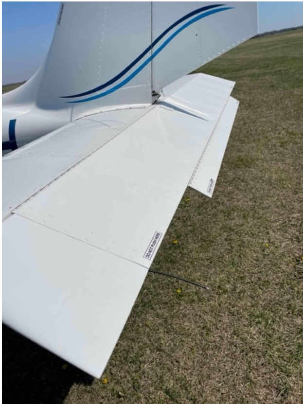
Full span elevator with electrically actuated central trim tab.
