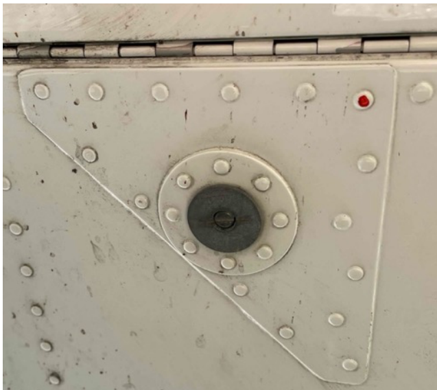
Main tank fuel drains just forward of the flap hinges.
