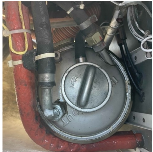
Rotax oil filler cap. (Where's the dipstick?)
