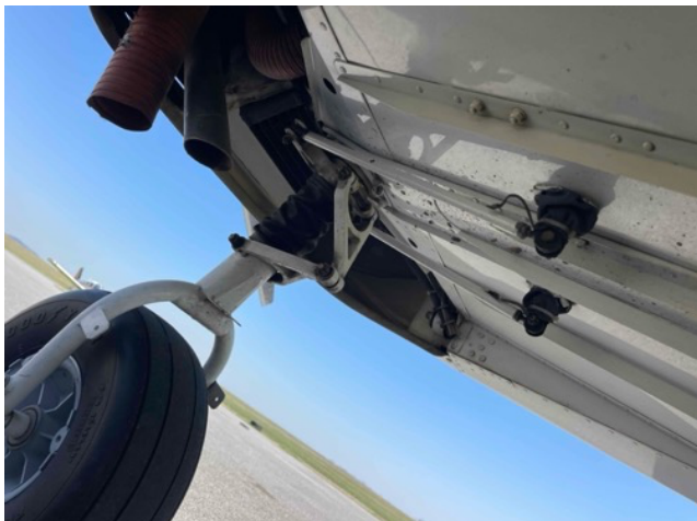
Nosewheel steering direct connections to rudder pedals but no gascolator drain.
