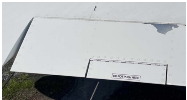
Electrically actuated aileron trim tab.
