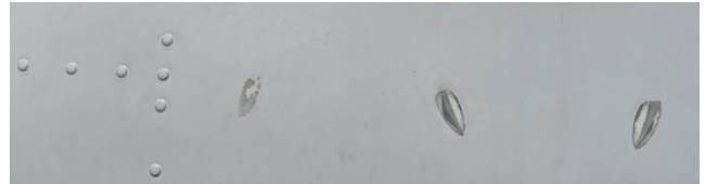
Adhesive mounted vortex generators. (One's missing. So how many do we need???)
