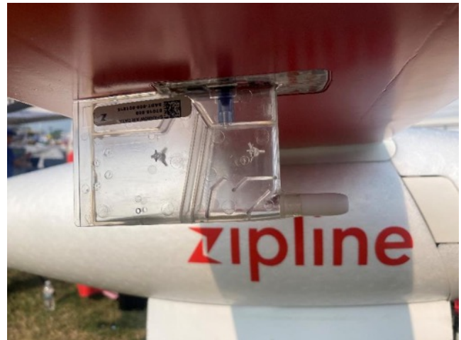
I'm probably the only person on the whole field who would get excited about this. This is the Zipline drone which has been used in Rwanda to deliver medications and for missions at several other locations. I looked at the Pitot tube and immediately recognized the baffles which are used for water separation to keep water out of the Pitot system.
