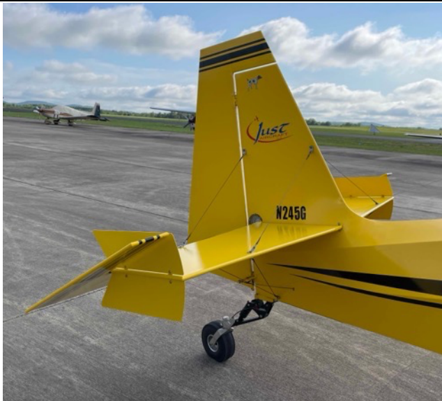
Here's a new one. "Fences" on the horizontal stab, inboard of the elevator aerodynamic counterbalance. (Zurg note: Flight test EAAers – have any of you seen this configuration before?)
