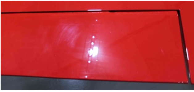
This Mystery Ship aileron is a beautiful piece of craftsmanship. Remember, this is fabric and dope over wood/metal.
