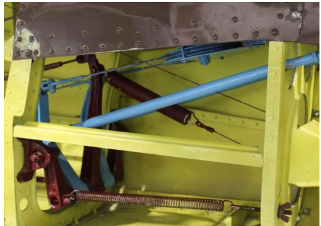
The simplicity of the "analog" mechanism that mixes pitch and yaw inputs to the two tailplanes.
