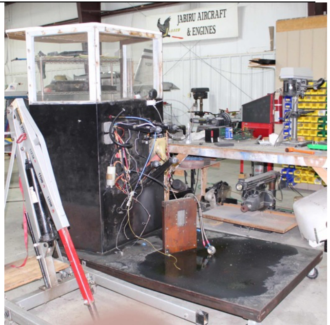
Arion's portable engine test stand. (Hum, this could bring a whole new meaning to the term “racing the engine on a test stand”. ;-)
