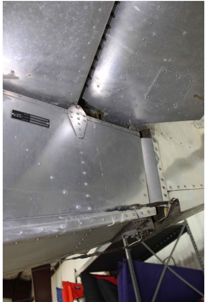
Zenith from 2 feet. “Ouch, that tail tiedown and rudder pivot bearing don’t look good AT ALL!”
