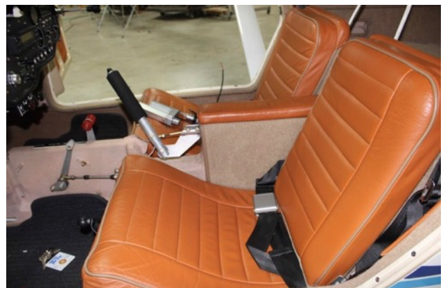
Jabiru J430 side stick (designed to doubly confuse Cessna pilots and instructors who are used to flying left hand in the left seat, and right hand in the right seat.)
