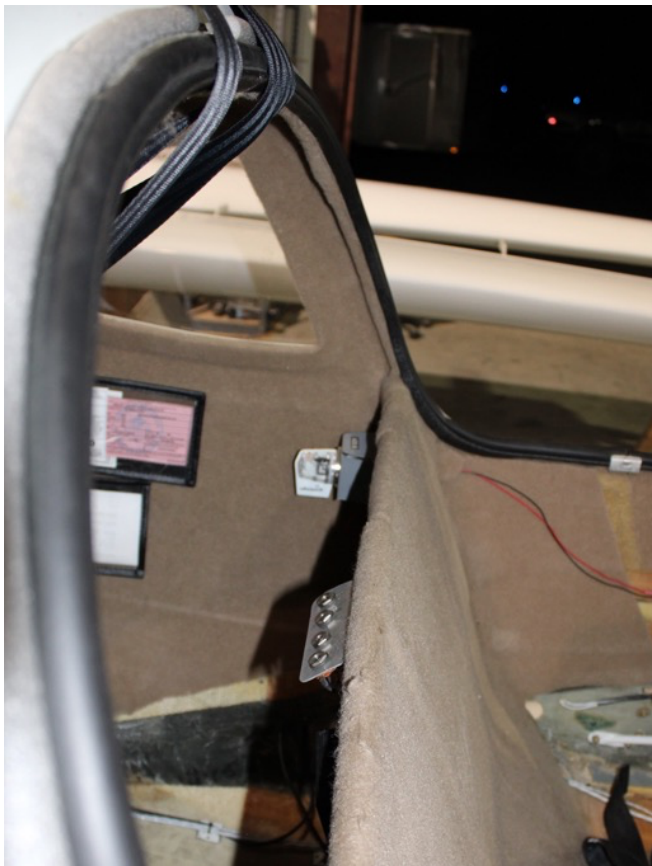
ADSB-out tail beacon stealthily hidden behind the seat.
