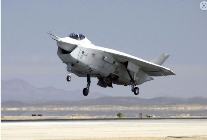
The newest aircraft on this list, the Boeing X-32 was designed for use by the Joint Strike Fighter (JSF), only to lose out to the Lockheed Martin X-35. Despite taking its first flight in 2000, the demonstrator's origins date back to 1993, when the Defense Advanced Research Projects Agency (DARPA) launched the Common Affordable Lightweight Fighter (CALF) project. A number of concepts were presented, including the X-32.
