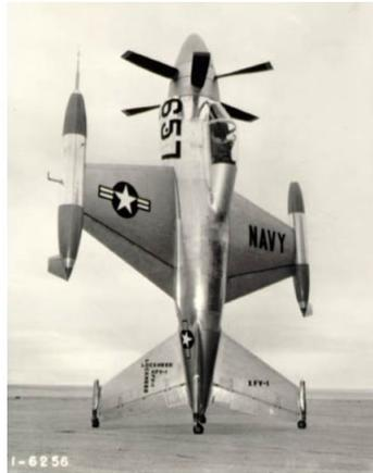
That's not a rocket you're looking at – it's the Lockheed XFV Salmon, an experimental aircraft designed to takeoff and land vertically. Intended to be flown by the US Navy, the plan was for the fighter to be used in the defense of convoys, but it never left the prototype phase. We'd like to say we can't understand why, but we think the reason is pretty obvious in this instance.
