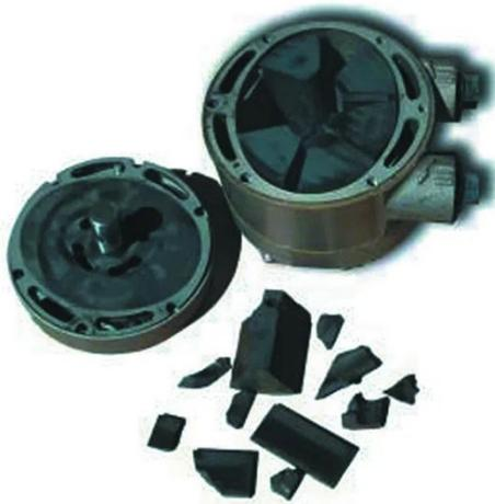
Vacuum pumps fail catastrophically and mean that IMC ops will rely on a pilots partial panel skills unless there's a backup attitude indicator.
