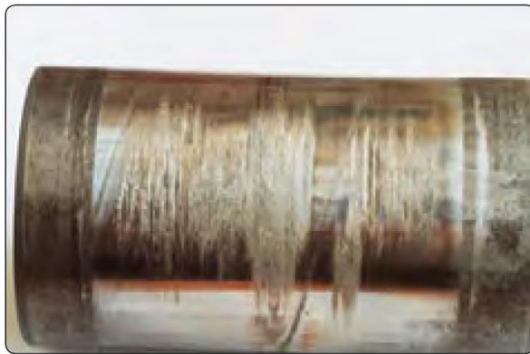
Figure 13-64. Galling is caused by rubbing of mating surfaces. The metal gets so hot it welds, and the surface metal is destroyed as the motion continues and pulls the metal apart in the direction of motion.
