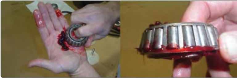
Figure 13-45. Packing grease into a clean, dry bearing can be done by hand in the absence of a bearing grease tool. Press the bearing into the grease on the palm of the hand until it passes completely through the gap between the rollers and the inner race all the way around the bearing.
