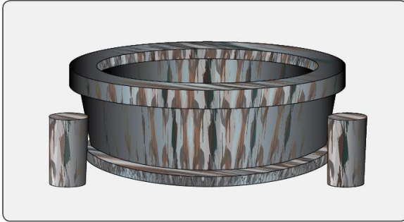
Figure 13-70. Etching and corrosion is caused when water, and the damage caused by water, penetrates the surface treatment of the bearing element. It appears as a reddish/brown discoloration.
