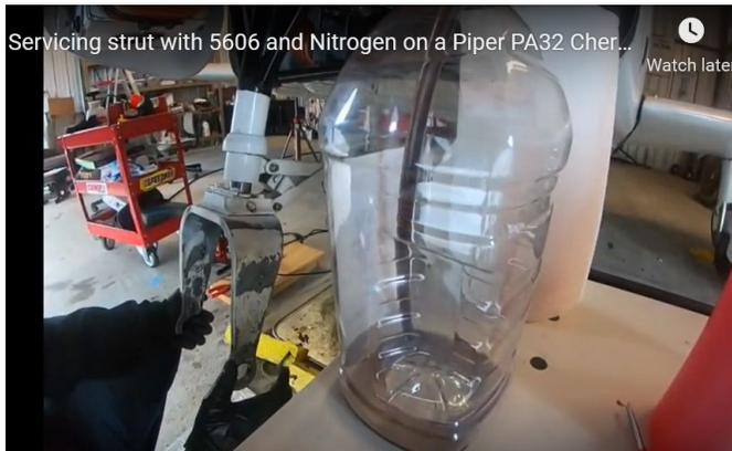
6. Connect clear hose or tubing To the Valve Core Stem
