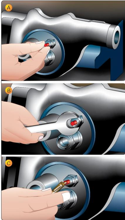
2. Remove the cap from the air servicing Valve
