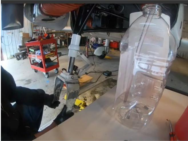
7. Push Strut Up, pushing old Hydraulic Fluid out of the strut into the jar Cycle a couple of times
