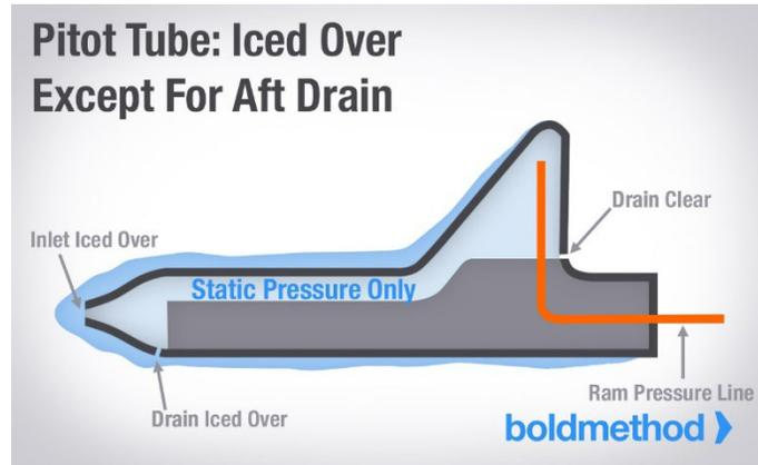
In this situation, the pitot tube becomes a relatively inaccurate static port.
