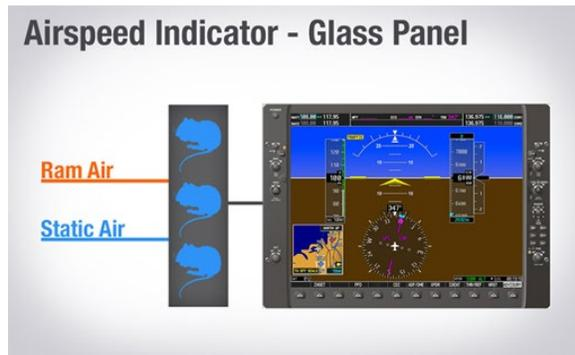
Glass-panel systems use digital sensors, which compare the ram and static air to indicate your airspeed.
