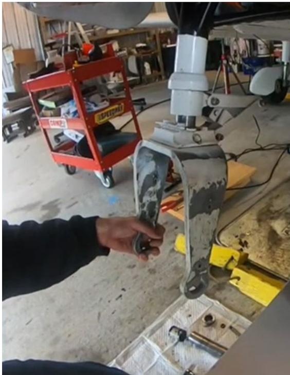
11. Finally compress the strut all the way and then pull strut back 1/4 inch
