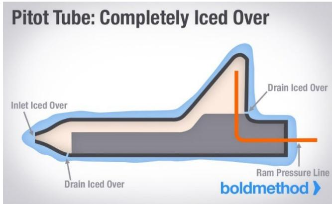
In this case, the ram pressure is trapped. As long as you stay at the same altitude, your airspeed freezes as well.
