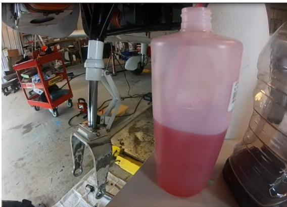
8. Connect clear hose or tubing to Valve Core Stem
