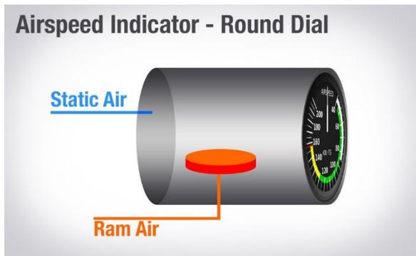
The traditional round-dial instrument uses an aneroid wafer filled with ram pressure, inside a case filled with static pressure.
