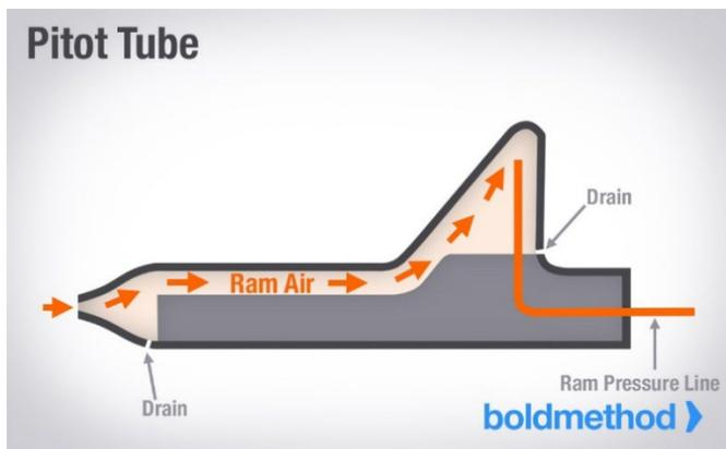
Ram air enters through the front of the tube, flows to the back of the chamber, and flows through plumbing to your airspeed indicator.
