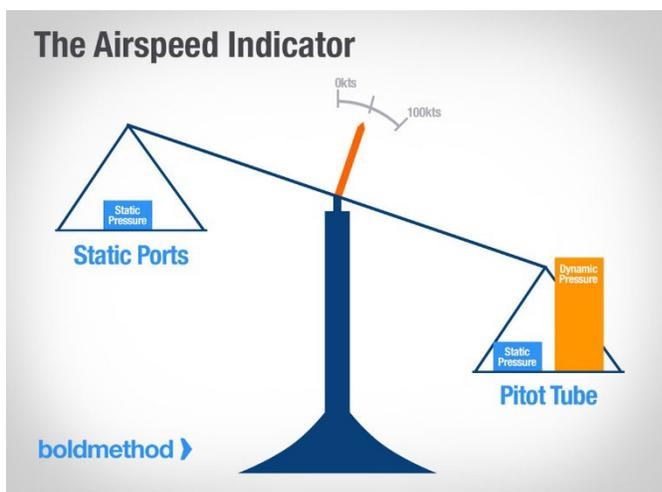
Your airspeed indicator is really a scale, which compares the static pressure from your static ports to ram pressure (static + dynamic) from your pitot tube. The two static pressures cancel each other out, and you're left with dynamic pressure.
