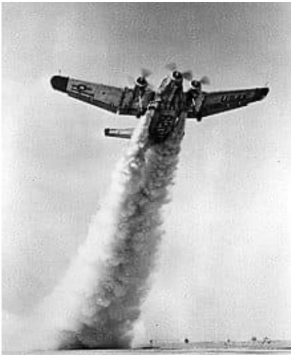
Six JATO (jet-assisted take off) bottles could be used to enable a fully loaded 40,900 lb YC-125 to take off in 500 ft
