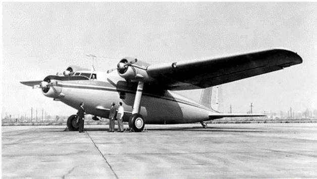
The Pioneer was unlike any aircraft that Northrop had built. The N-23 Pioneer was a trimotor, high-wing aircraft of all-metal construction. Its robust fixed landing gear, with long struts, enabled the aircraft's use on unimproved runways. To allow for short-field operation, large flaps made up 80% of the wing's trailing edge.
