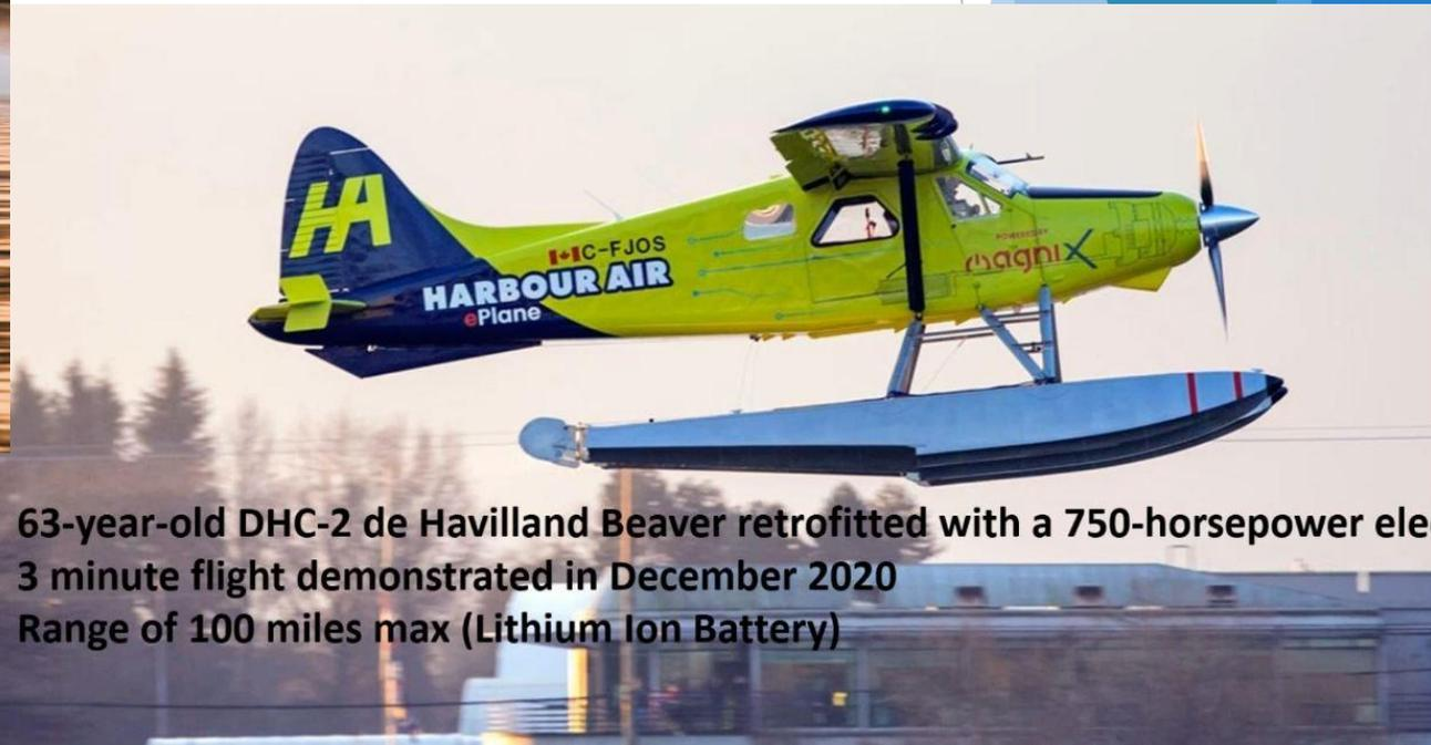
63-year-old DHC-2 de Havilland Beaver retrofitted with a 750-horsepower electric motor. A 3 minute flight demonstrated in December 2020
