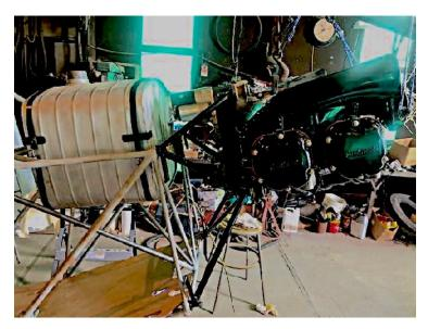
I added Grove disc brakes, a C-85 continental engine in place of the original Franklin that was long gone. Also installed a B&C light weight starter along with a Lithium-ion light weight battery.
