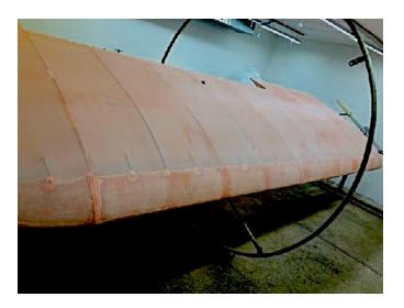
The covering system is a multi-step Poly Fiber as that is what I am familiar with. The pictures of the wing is the complete covering process. The fabric is glued on then shrank with a regular electric clothes iron in 3 stages, increasing the heat
