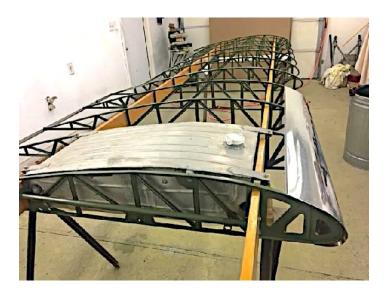
I also installed is a 12-gallon wing tank in the left wing that feeds into the 12-gallon fuselage tank by opening a valve
