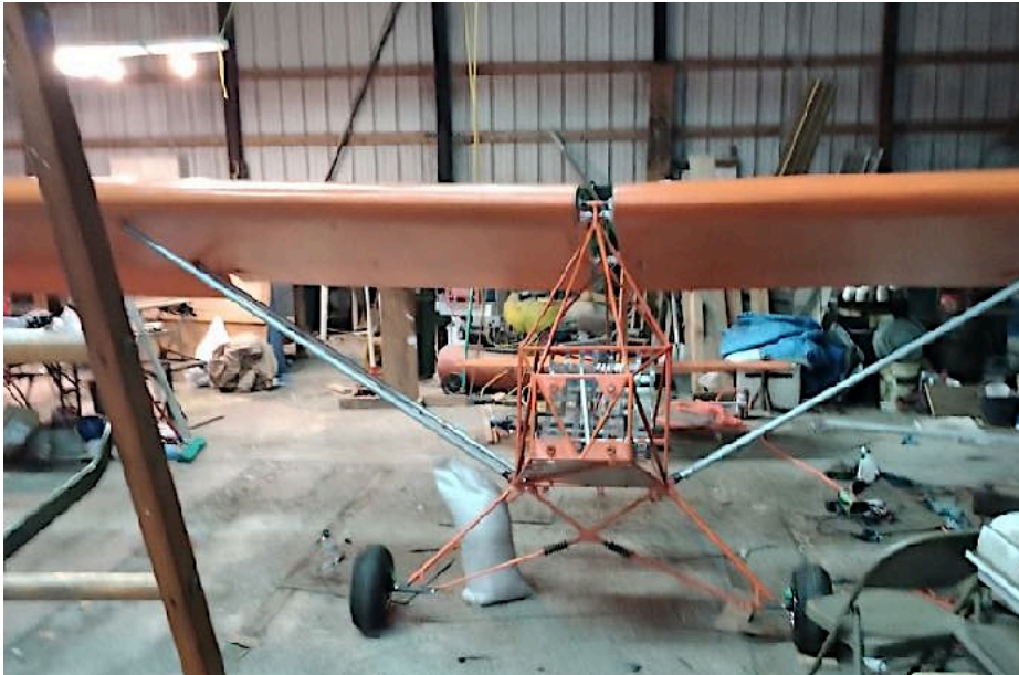
Mounted wings to explore methods for folding wings for storage.
