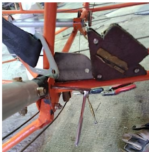
Welding seatbelt brackets
