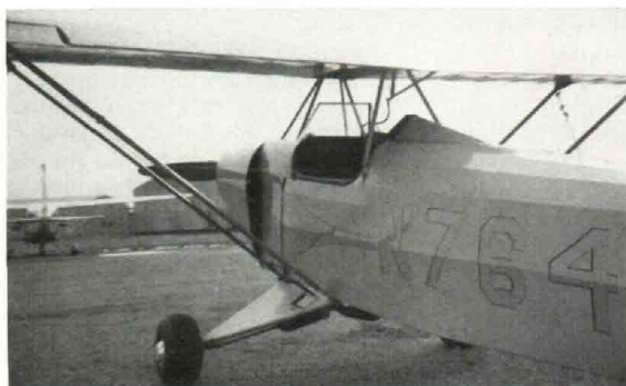
The wing panels were adapted from an original set built for the Price "Parasol." The rear opening of the cowl allows enough room for checking the gas and oil.
