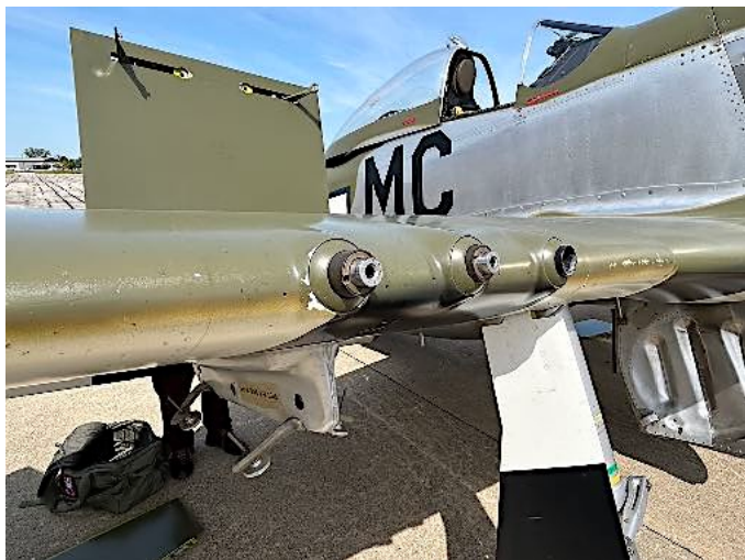
The aircraft still has the original armament of six 50 caliber machine guns in the gun bays
